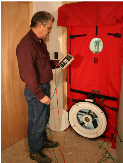
The author performing a blower door test
